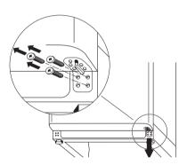
3. Remove the door fitting from the door hinge bracket (1, 2). Move the hinge bracket pivot from the right to the left hand hole (3). Place the door fitting supplied on the hinge bracket pivot (4, 5).
